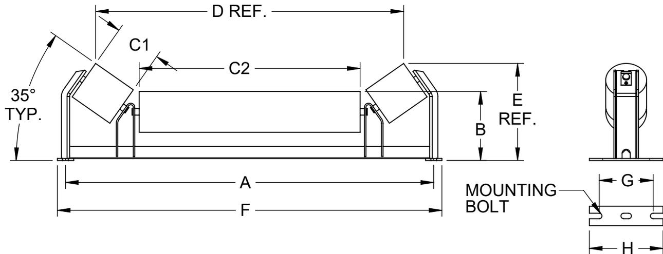
**CEMA C 35° PICKING TROUGH IDLER 4" DIAMETER ROLLS**
