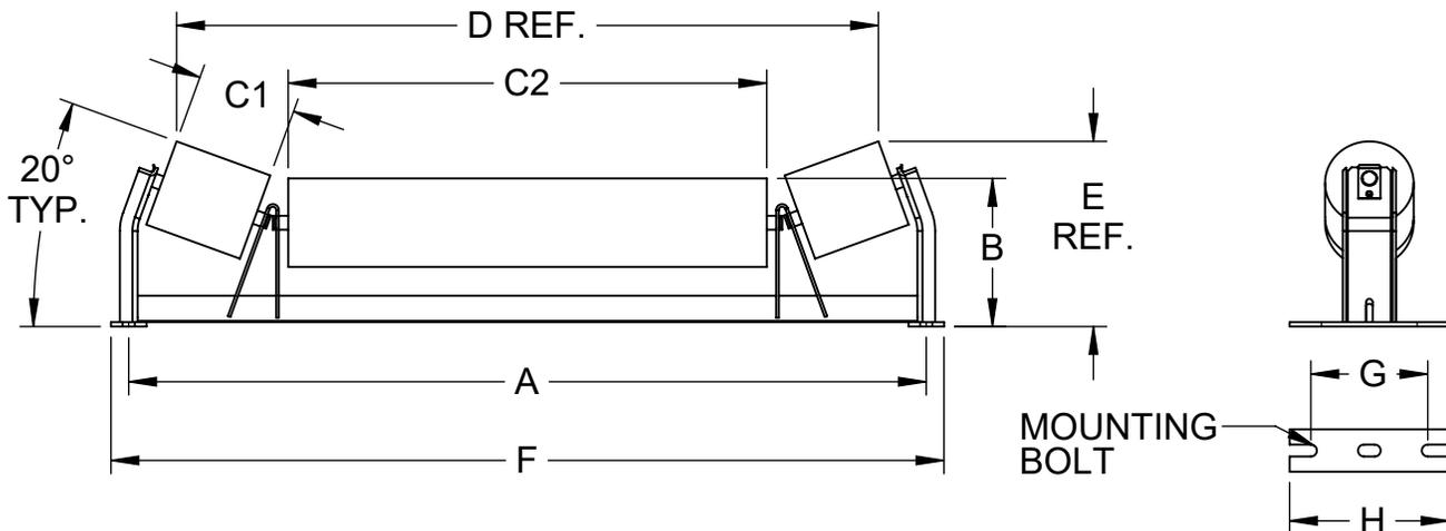
**CEMA C 20° PICKING TROUGH IDLER 4" DIAMETER ROLLS**
