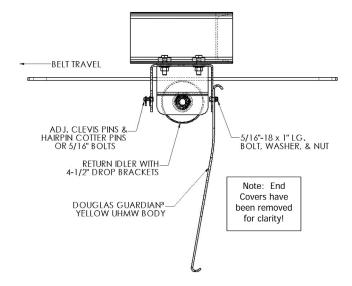
The Douglas Guardian<sup>3</sup> Side Shields are designed to allow visual inspection of the return roll assembly without removing any parts! The Side Shield is made from 100% flexible UHMW and can be left as shown or tucked in at the bottom edge. A tab is provided on the bottom of each Side Shield and can be adjusted to engage with the bottom slot on the
